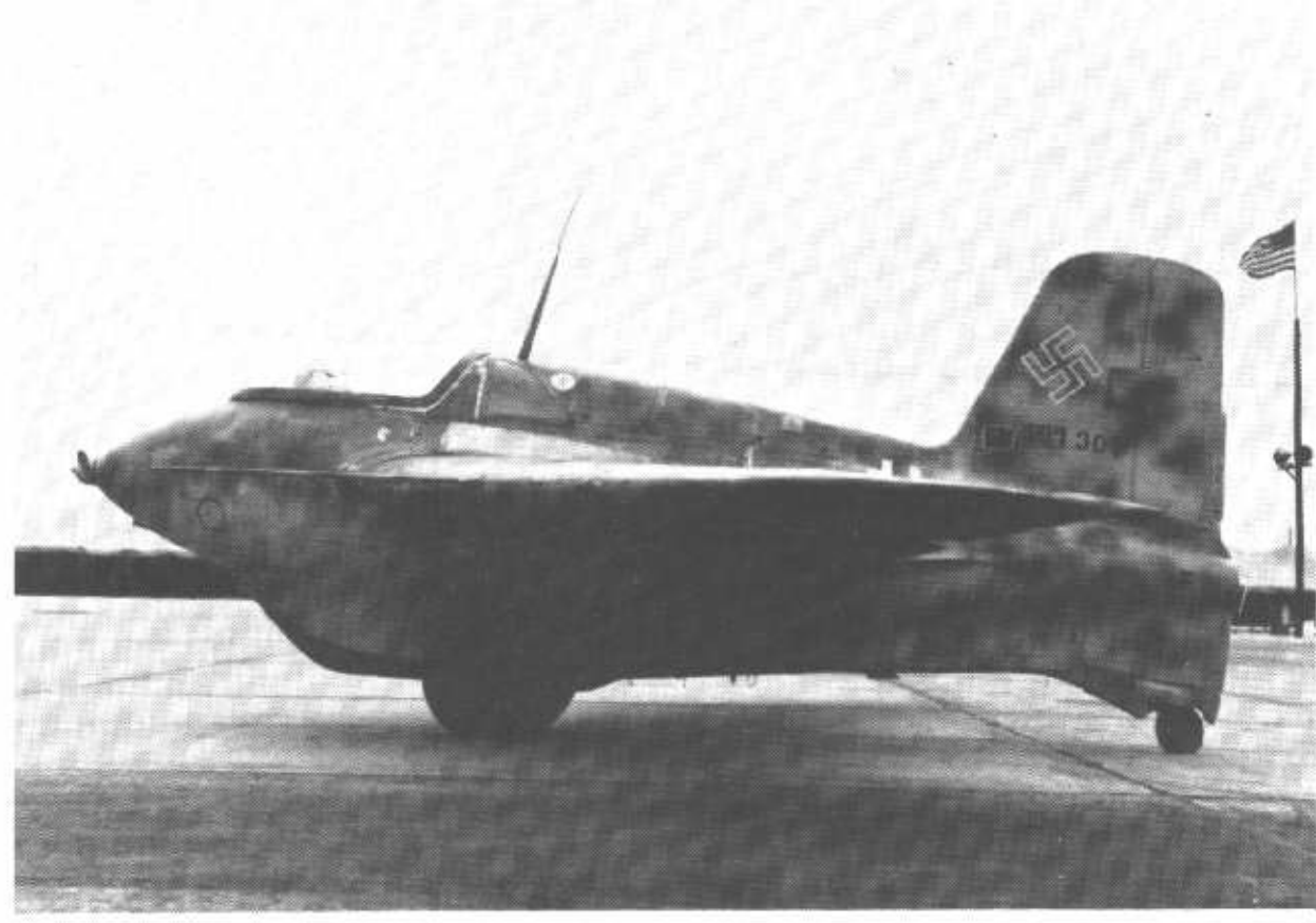
Japan received manufacturing rights and production drawings from Germany for the Messerschmitt Me 163. Approximately four of these Mitsubishi J8M1 Shusui rocket fighters were built for the Navy, and one as the Ki.200 was for the Army. These were reasonable copies of the Me 163, but material substitutions had to be made in the airframe as well as the Walter rocket engine. A larger version known as the Ki.202 was in the planning stage.
